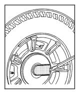
Remove the center cap by placing the flat end of the wheel wrench in the slot on the wheel and gently pry the center cap out.
